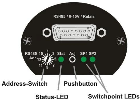
The VSM is equipped with a status LED which signalizes the following operational states:
